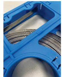
**Step Two** – Once recoiled and loose, feed the end back through the indicated slot below. Again, you may need to shake the case to move the strapping towards the opening.
