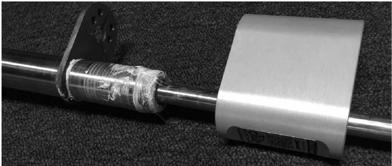
29. Using a 13mm socket, tighten the gauge housing bolts.
