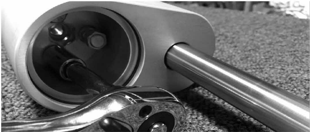
29. Using a 13mm socket, tighten the gauge housing bolts.
