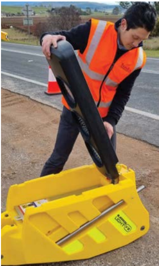
Raise the light head You will hear clicking going up.
