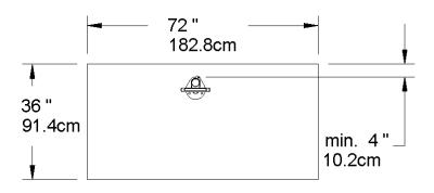
The minimum space requirements for High Security Bike Pumps are meant to allow a cyclist and their bike access to the pump.
