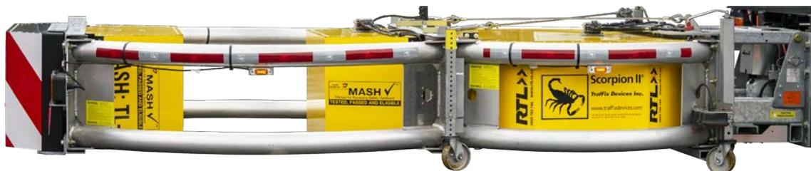
*This TMA is designed as a crash attenuator only. It must not be used as a mobile barrier or for any other purpose outside of crash attenuation and should only be deployed at speeds up to 50 km/h. Any use outside these conditions will void the warranty.*
