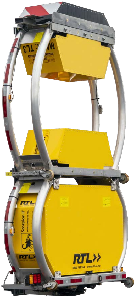
The C-90 TMA is stored in the vertical position only
