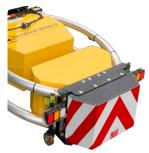
The Metro-SLIM provides full width impact protection by redirecting the impacting vehicle with its patented curved aluminium tube frames and energy absorbing modules. The curved aluminum tubes provide protection against nuisance impacts while providing re-directional capabilities along the entire length of the TMA.
