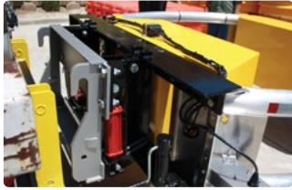
1. Back up truck to Fast-Trak SwiftConnect™
