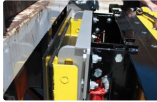
2. Align mounting hooks over connection bars & lower into place
