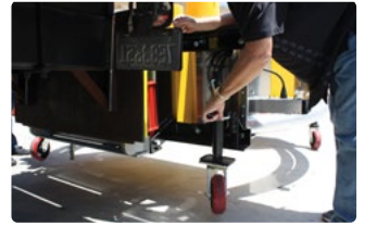
4. Crank down and insert lock pins
