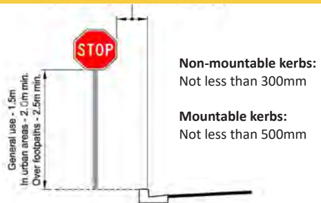
Figure 7.2 Lateral and height clearances for regulatory and warning signs in un-kerbed roadways
