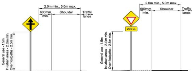
Figure 7.2 Lateral and height clearances for regulatory and warning signs in un-kerbed roadways
