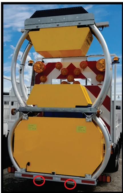
Fig.3 Access the grease points.
