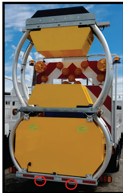
Fig.3 TMA in the stored position and where to access the grease points.
