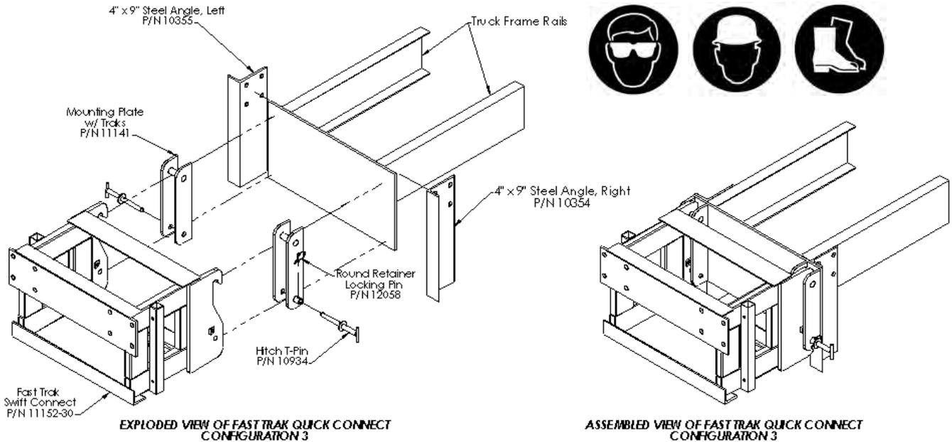
Figure 5: Exploded and assembled view of Configuration 3.
