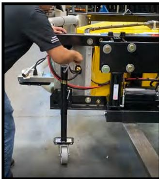
11. Lower the swivel jacks so the TMA is no longer supported by the forklift.
