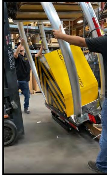
5. Once the drop jacks can safely be reached, do not lower the TMA any further. Extend the drop jacks so that the yellow painted edge is aligned with the bottom of the drop jack mounting bracket. Secure the drop jacks in place with the safety snap. Continue to lower the TMA until the drop jacks have reached ground level.
