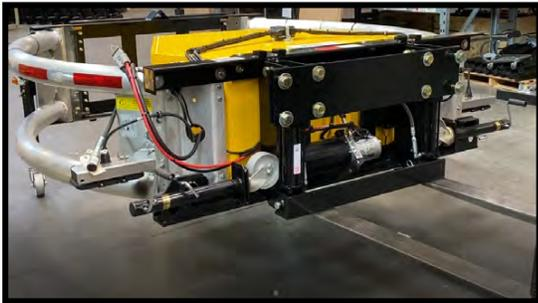
10. Move the lifting straps towards the Back-up of the TMA and lift, using a forklift, until the unit is level.
