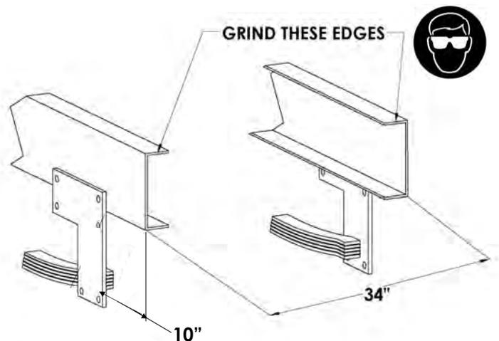
2. A backing plate (33" x 10") should be centered on the back of the truck frame. Note where the frame will be welded to the plate and grind the plate in this location. Tack weld the rear plate into position and make sure that the rear plate is positioned vertically at 90° to horizontal. Continue by welding the inside of the frame end to the plate.
