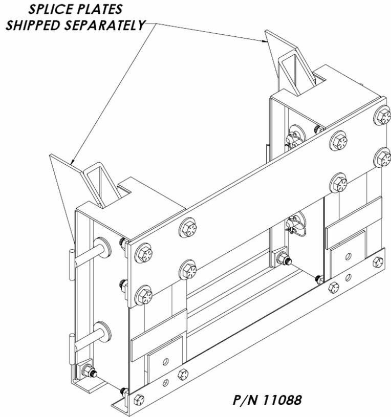
4. Once the TMA is rolled towards the back of the host vehicle, tack weld the tubes in place at the outermost and innermost four corners where the tubes touch the frame. This image below illustrates ideal tack welding locations to hold the tubes in place.
