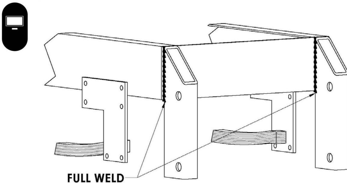
6. Position the splice plates, as shown here in this figure below, against the sides of the frame and the vertical tubes. Mark on the plate the position of two holes for  $\frac{3}{4}$ " bolts. Drill these holes in the plates and the frame. Weld the edge of the plate to the vertical tube. The truck frame weld areas should be spray painted to prevent rust.
