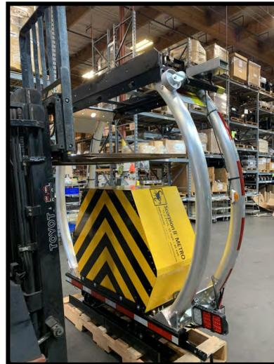
3. Using a forklift, lift the TMA off the pallet. **CAUTION:** Be sure the drop jacks are facing the forklift before lifting the TMA. Once the TMA is safely off the pallet, remove the mounting brackets that are on the pallet.
