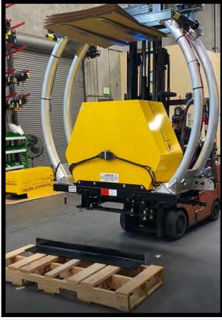
6. Lift the TMA off the pallet using a forklift.
