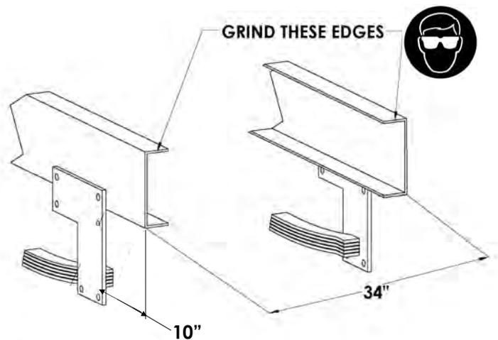
2. Mount the Backing Plate (P/N: 10353) onto the backup of the TMA as shown in this figure (right). Mounting the backing plate onto the TMA will simplify the alignment process when mounting the backing plate onto the truck frame of the host vehicle.
