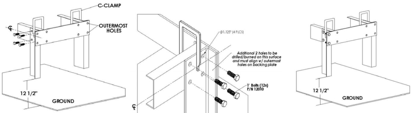
7. Weld the angles in place at the rear of the angle. Refer to the figure below for proper welding locations.
