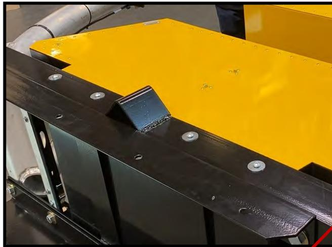
Appropriate to use either a Ratchet and Socket or Impact Wrench when tightening bolts.
