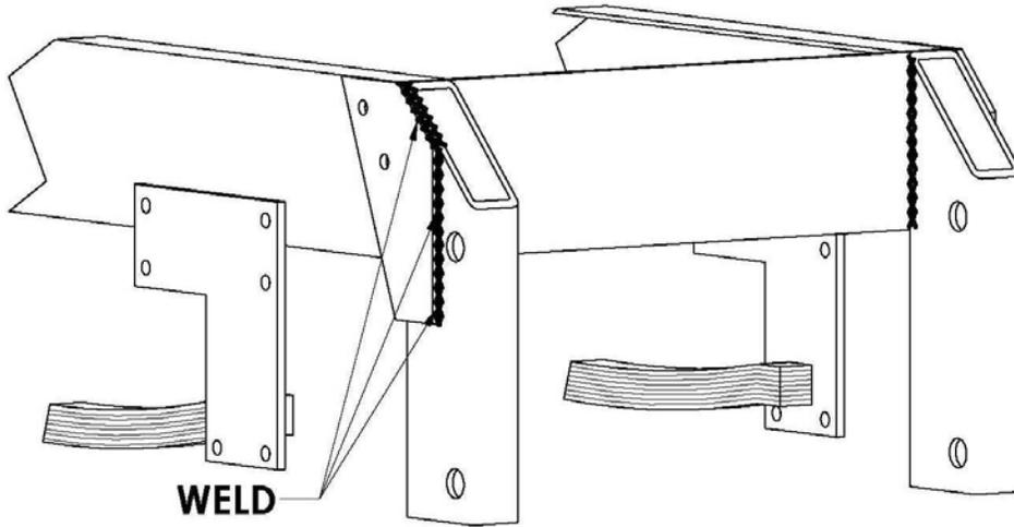
7. After the splice plates have been welded on the tubes, Install the four  $\frac{3}{4}$ " bolts in the designated holes that were drilled into the plates to reinforce the splice plates as well as the tubes..
