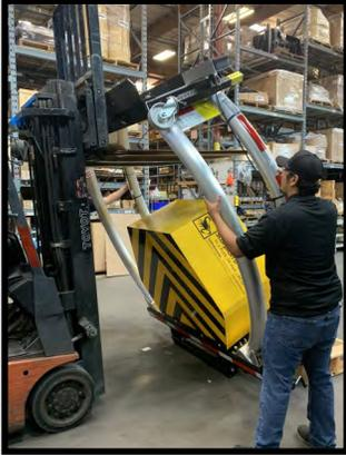
8. Reposition the TMA on the edge of the pallet.
