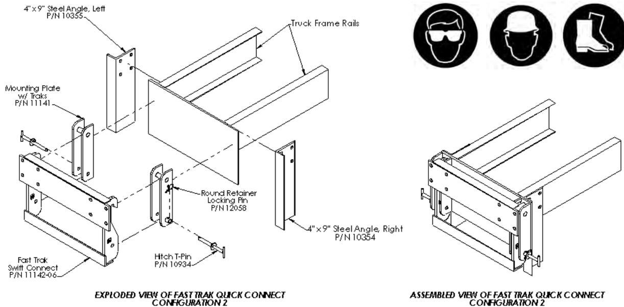
Figure 4: Exploded and assembled view of Configuration 2.
