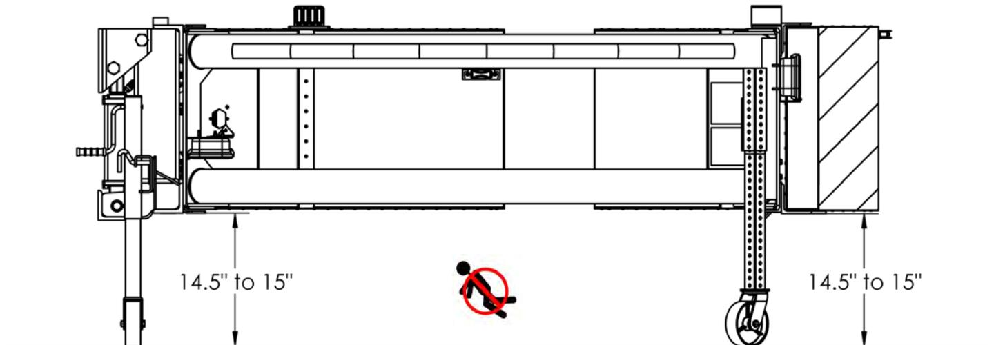
4. With the jacks deployed, roll the deployed TMA to the rear of the host vehicle and align the TMA centerline with the vehicle, as shown in the following figure. The backing plate that is bolted onto the TMA (See step 2) should be flush with the ends of the truck frame.
