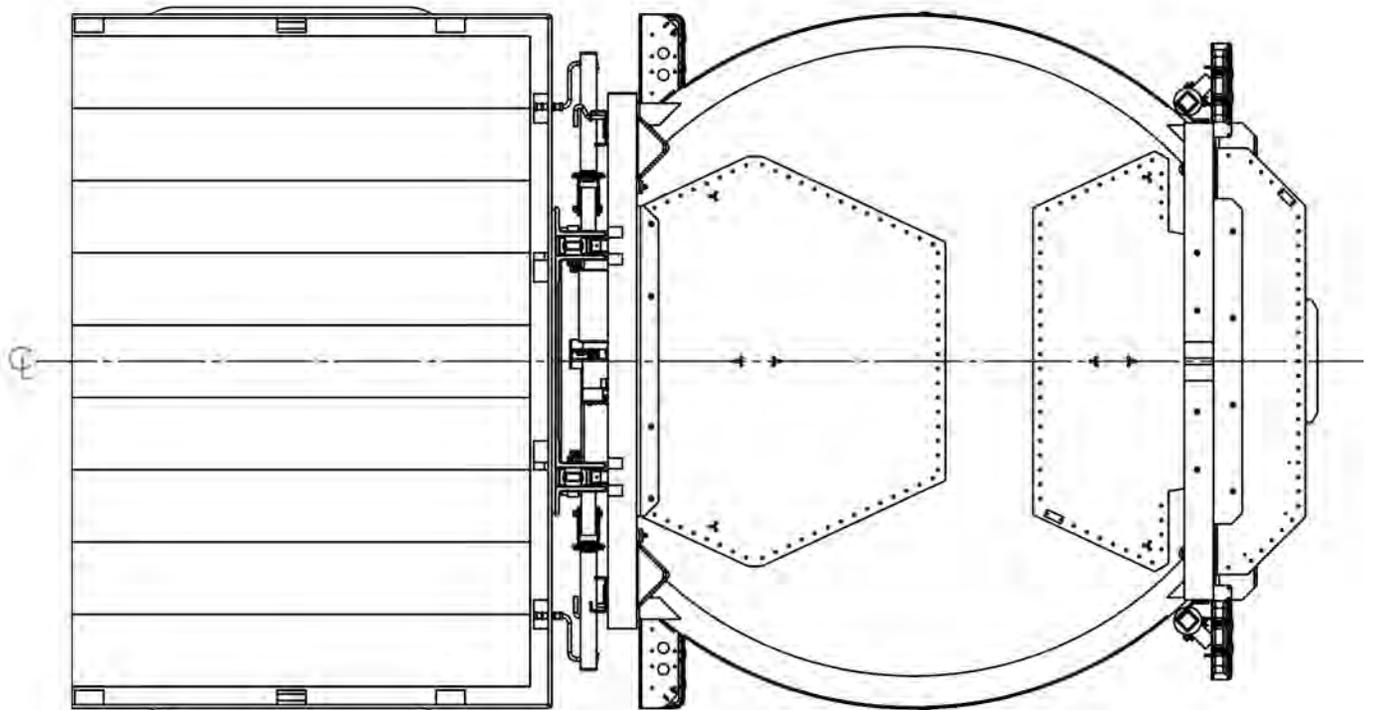
5. After proper confirmation of the backing plate being level and 90° to the horizontal surface, deploy the drops jacks and unbolt the TMA from the backing plate that is already tacked onto the host vehicle. Fully weld the backing plate on both the inside and outside of the frame rails. Proper welding locations are specified in the figure below:
