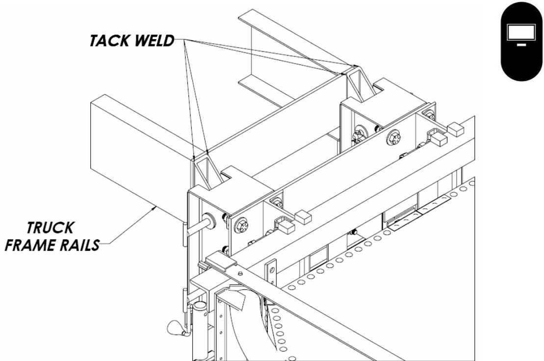
5. Remove the four 1" bolts from the vertical tubes and roll the TMA rearward to pull the extension frame free from the vertical tubes. Fully weld the tubes in place on all four sides where the tubes touch the frame and the back plate. Refer to following figure for details.
