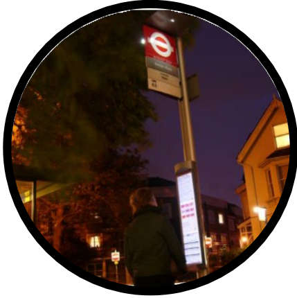
LED Edgelit technology to backlight timetable
